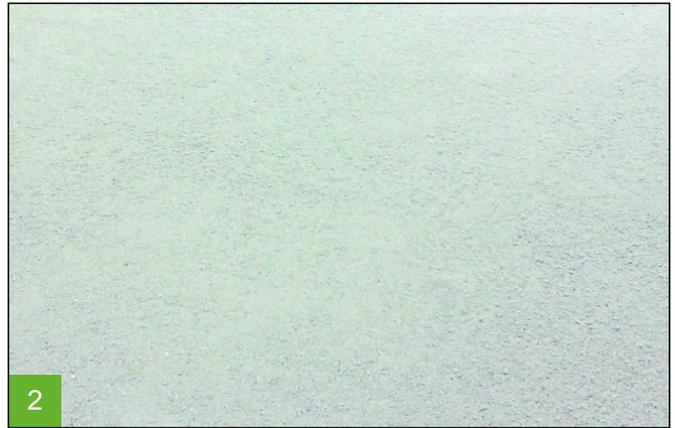
**Cement screed (CT)**; This very common screed type is used in all types of buildings. Cement screeds have little susceptibility to moisture, but in the first few weeks after installation show a distinct shrinkage curing behaviour of around 0.5 mm/m.
