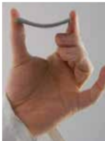
S2 Verformung ≥ 5 mm
